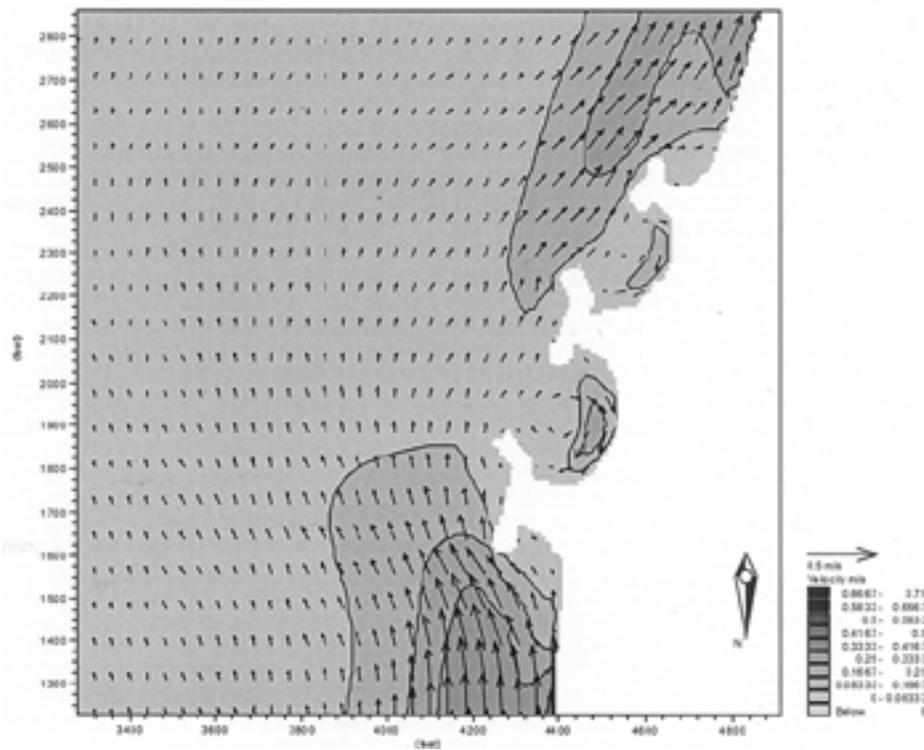
**FIGURE 7 : Results of Current Model-Proposed Configuration**
