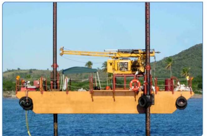
A marine geotechnical investigation is oftentimes required to confirm a project site's suitability to accommodate cruise pier structures and any required dredge/fill operations. A jack-up barge is typically utilized as a stable platform for offshore drilling.
